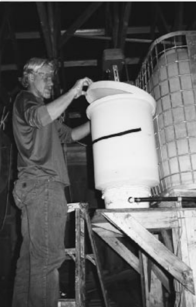
PRODUCTION COORDINATOR CHRIS RILEY OPENS THE LID OF A COOLED DOWN REACTION VESSEL. THE HEAVIER GLYCERIN SETTLES ON THE BOTTOM OF THE VESSEL, AND THE LIGHTER BIODIESEL LIES ON TOP.
